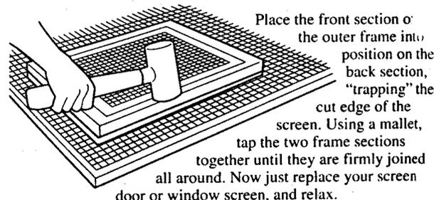
Place the front section of the outer frame into position on the back section, "trapping" the cut edge of the screen. Using a mallet, tap the two frame sections together until they are firmly joined all around. Now just replace your screen door or window screen, and relax.
