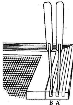
Now determine if your screen door or window screen is metal or fiber. If it is metal, cut around the entire edge of "A" with a small, sharp knife, using the grooves as a guide. If your screen is fiber, cut around the entire edge of "B", using the grooves as a guide. Be sure to hold the Pet Screen Dor frame solidly in place with one hand so it doesn't move during cutting. Remove the cut-out portion of the screen.
