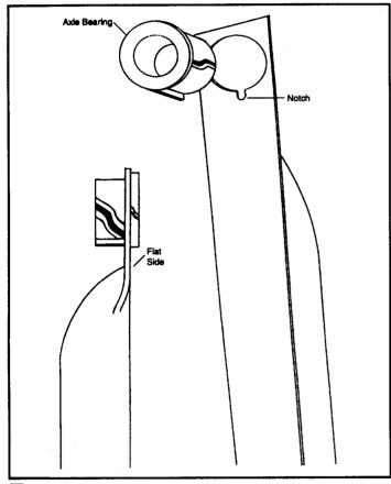
Install axle bearings to both lower handles.
