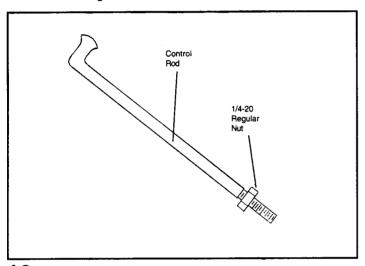
16 Install (1) 1/4-20 regular nut (not a locknut) on to control rod as shown.
