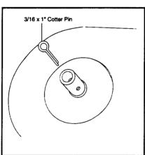
Install coast wheel to axle using outside pin hole. As shown, insert 1" cotter pin through axle. Bend with pliers to prevent pin from falling out.
