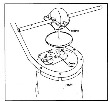
6 Install gear box by inserting the pinion shaft into hole in center of hoppers bottom.
