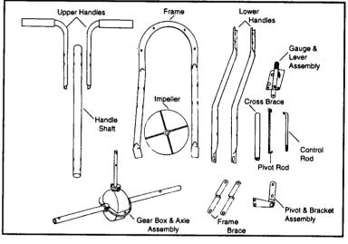
Remove and identify loose parts from carton and bag.
