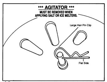
Insert large hair pin clip to pinion shaft on inside of hopper. NOTE: Position of flat side of hair pin clip. This pin should be installed as shown.
