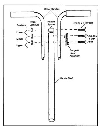
NOTE: BEFORE INSTALLING GAUGE AND UPPER HANDLES TO HANDLE SHAFT, UPPER HANDLES FEATURE THREE POSITIONS FOR OPERATOR'S COMFORT. If operator chooses middle or upper positions, use handle spacer in hole nearest to handle grips. Insert 1 1/2" bolt through upper handle, then through handle spacer through other upper handle. DO NOT TIGHTEN LOCKNUT YET. TIGHTEN THIS NUT LAST. Install gauge & lever using (2) 1 3/4" bolts. Be sure gauge is on left hand side. Tighten locknuts to gauge first. TIGHTEN NOW.
