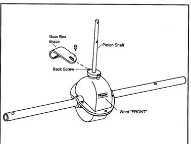
Remove screw from back side of gear box assembly and install gear box brace as shown. **NOTE:** Gear box brace should be in line with pinion shaft.
