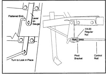
Install flattened end of control rod in to lever on gauge as shown. Turn to lock in place. Next push lever forward to setting "0". Align control rod up with hole in pivot bracket, pull lever backward to insert control rod through hole in pivot bracket. Now install 1/4-20 regular nut on to control rod. **DO NOT TIGHTEN NUTS YET.**
