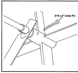
9 Slide axle bushing over axle and into axle bearing to both sides as shown.
