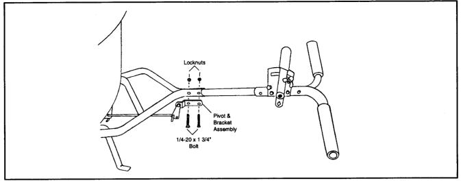
Install handle shaft to lower handles and pivot & bracket assembly as shown. Using (2) 1 3/4" bolts and (2) locknuts. Tighten bolts and nuts now.
