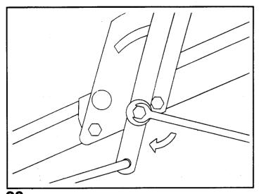
Tension on the flow control lever may be adjusted by tightening or loosening the tension nut as shown.
