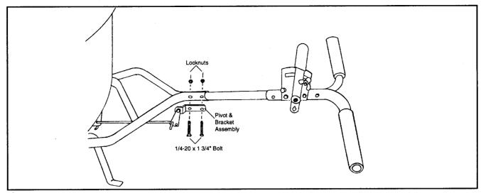
15 Install handle shaft to lower handles and pivot & bracket assembly as shown. Using (2) 1 3/4" bolts and (2) locknuts. Tighten bolts and nuts now.
