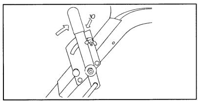
Pull lever back to setting "30" as shown. Next push pivot & bracket forward so that the shut off plate in the hopper is in the full open position. REMEMBER SETTING "30" ON THE FLOW CONTROL LEVER MUST PLACE THE SHUT OFF PLATE IN THE FULL OPEN POSITION TO BE PROPERLY CALIBRATED. Now tighten the nuts against the pivot bracket to prevent change in calibration.
