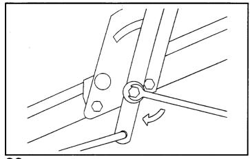
Tension on the flow control lever may be adjusted by tightening or loosening the tension nut as shown.
