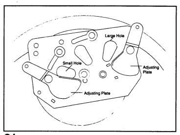
For normal operation both plates should be full open. To reduce flow to the left side, partially or completely close the plate over the rear (large) hole.
