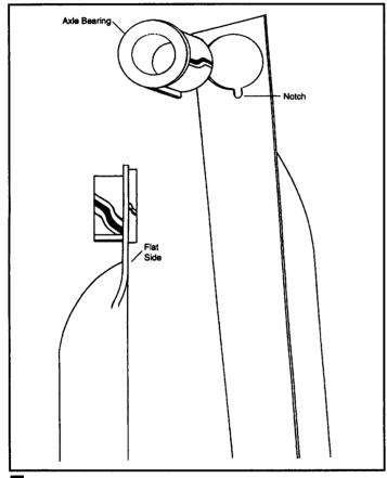
Install axle bearings to both lower handles.
