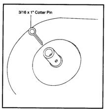
11 Install coast wheel to axle using outside pin hole. As shown, insert 1" cotter pin through axle. Bend with pliers to prevent pin from falling out.
