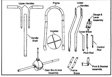
2 Remove and identify loose parts from carton and bag.
