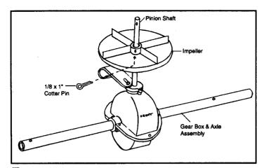
Install impeller onto pinion shaft. Insert 1/8" x 1" cotter pin through impeller then through pinion shaft. Use hole nearest gear box. Spread cotter pin to prevent from falling out.
