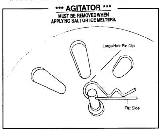
Insert large hair pin clip to pinion shaft on inside of hopper. NOTE: Position of flat side of hair pin clip. This pin should be installed as shown.
