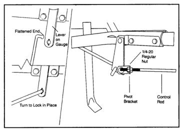
17 Install flattened end of control rod in to lever on gauge as shown. Turn to lock in place. Next push lever forward to setting "0". Align control rod up with hole in pivot bracket, pull lever backward to insert control rod through hole in pivot bracket. Now install 1/4-20 regular nut on to control rod. DO NOT TIGHTEN NUTS YET.
