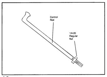
16 Install (1) 1/4-20 regular nut (not a locknut) on to control rod as shown.
