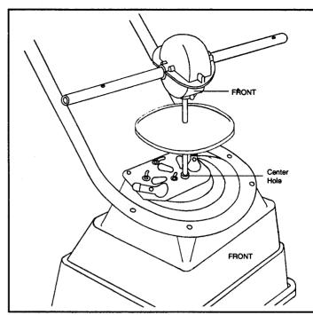
6 Install gear box by inserting the pinion shaft into hole in center of hoppers bottom.
