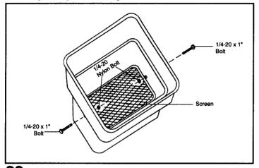
Install screen inside hopper. Fasten using (2) 1/4-20 x 1" bolts and (2) 1/4-20 nylon insert locknuts. Tighten now.
