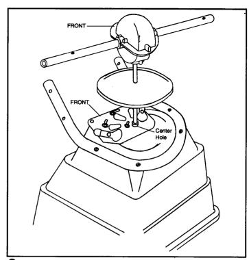
6 Install gear box by inserting the pinion shaft into hole in center of hoppers bottom.
