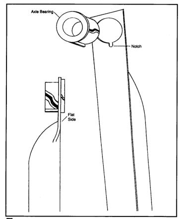
Install axle bearings to both lower handles.
