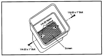
Install screen inside hopper. Fasten using (2) 1/4-20 x 1" bolts and (2) 1/4-20 nylon insert locknuts. Tighten now.
