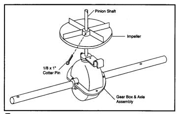
5 Install impeller onto pinion shaft. Insert 1/8" x 1" cotter pin through impeller then through pinion shaft. Use hole nearest gear box. Spread cotter pin to prevent from falling out.
