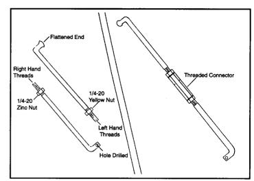
16 Install the 1/4-20 yellow left hand threaded nut onto the control rod with the flattened end. Install the 1/4-20 regular zinc plated nut (not a locknut) on the right threaded control. (Rod with drill hole).
