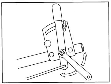
21 Tension on the flow control lever may be adjusted by tightening or loosening the tension nut as shown.
