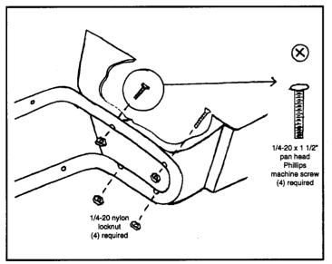
Position hopper on side. Install frame using (4) 1/4-20 x 1 1/2" pan head Phillips machine screws and (4) 1/4-20 nylon locknuts. First put bolts through holes inside hopper's bottom, then through holes in frame. Secure with locknuts. Tighten these locknuts now.
