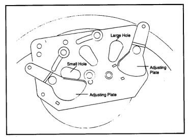
**22** For normal operation both plates should be full open.
