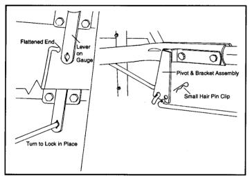
18 Install flattened end of control rod in to lever on gauge as shown. Turn to lock in place. Next insert round end of control rod in to pivot and bracket assembly. Secure in place using the small hair pin clip.
