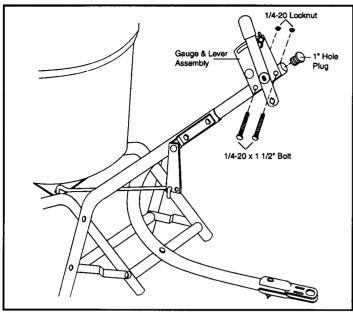
Attach gauge and lever assembly to control support using (2) 1/4-20 x 1 1/2" bolts and (2) 1/4-20 locknuts. TIGHTEN NOW.
