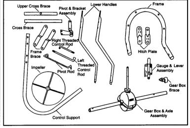
2 Remove and identify loose parts from carton and bag.
