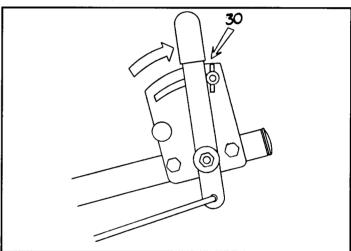
19 To calibrate the flow settings, put the flow control lever at setting 30. Adjust the length of the upper control rod by turning the threaded connector so that the shut off plate in the hopper is in the full open position. REMEMBER — Setting 30 on the flow control lever must place the shut off plate in the full open position to be properly calibrated. NOW tighten the nuts against the threaded connector to prevent a change in calibration.
