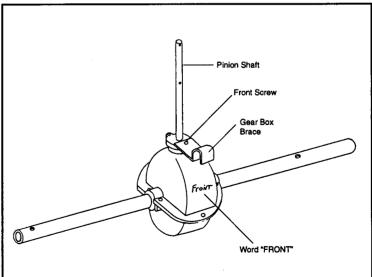
Remove screw from front side of gear box assembly and install gear box brace as shown. **NOTE:** Gear box brace should be in line with pinion shaft.
